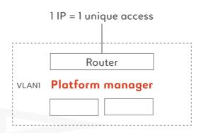
VLAN1 can access to VLAN2, 3 & 4 but not in the other direction. VLAN2, 3 & 4 are silos
